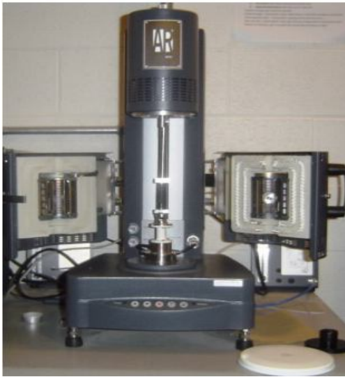
Figure 3-2. AR-2000ex Mechanical Test Station and Its Key Specifications
